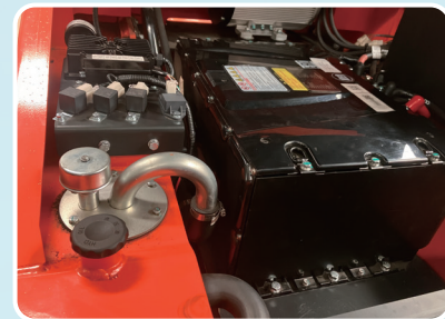
Convenient hydraulic oil level check.
